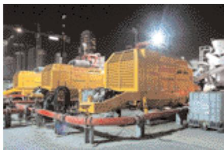
*Putzmeister-Betonpumpen BSA 14.000 SHP-D*
